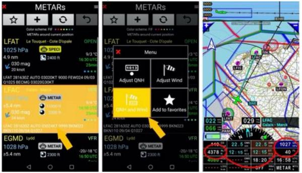
The local QNH has been modified, the value indicated in the flight level button FL is modified, while the GPS altitude remains unchanged.
