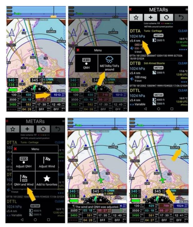
QNH value and wind are displayed, Fly Level altitude is adjusted.
