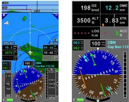
Artificial horizon and turn slip indicator are displayed on the **terrain** and on the **instrument** screens
