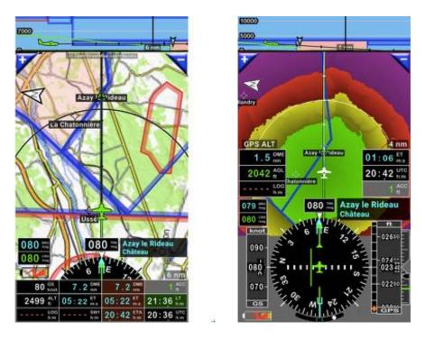
Glide path appears on vertical cut. Helpful function for pilots willing to control precisely their glide.
