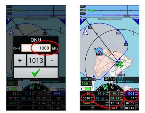
The local QNH has been modified, the value indicated in the flight level button FL is modified, while the GPS altitude remains unchanged.
