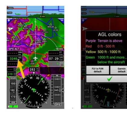
On moving map if aircraft is green, or if surface is green on terrain map, it indicates that altitude below aircraft is higher than 1 000 ft.
