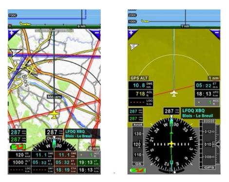
On moving map if aircraft is red, or if surface is red on terrain map, it indicates that altitude below aircraft is between 0 ft. and 500 ft.
